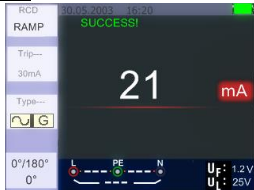
RCD Ramp – Measuring screen
