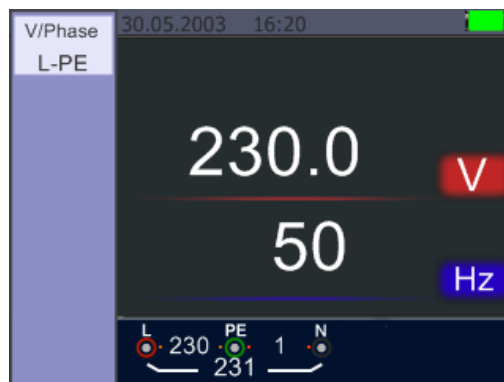
Screen while measuring Voltage and Frequency
